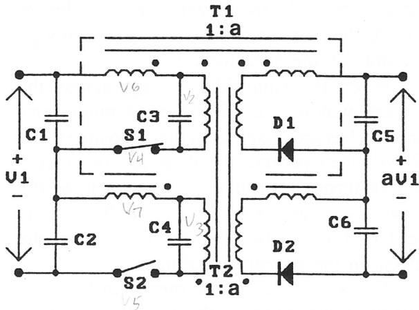
Figure 4. Split-tank Half-bridge Complementary-resonant Converter.
