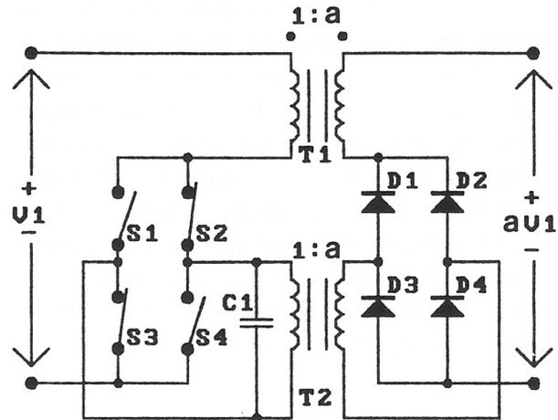
Figure 5. Full-bridge Complementary-resonant Converter.
