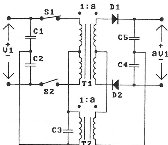
Figure 3. Single-tank Half-bridge Complementary-resonant Converter.
