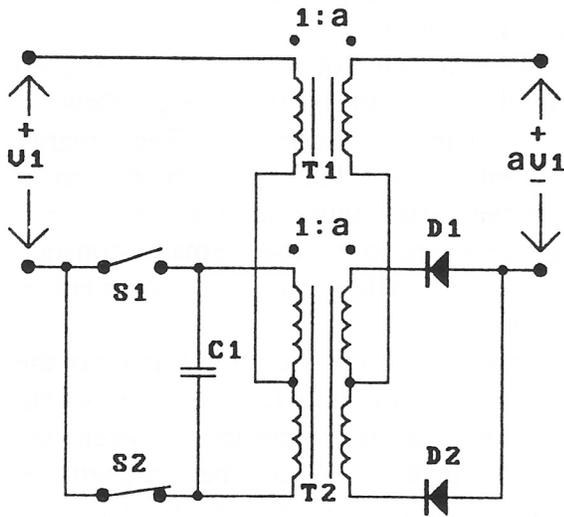
Figure 1. Center-tapped Complementary-resonant Converter.
