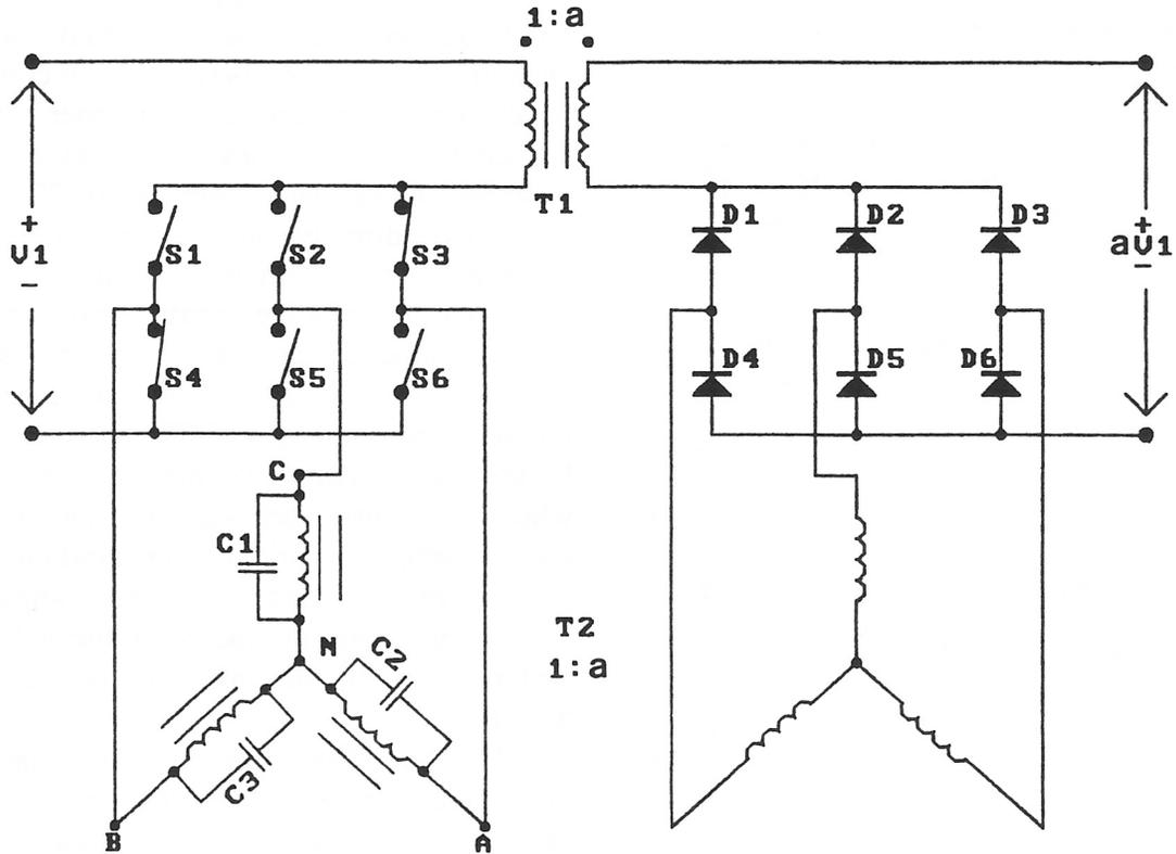
Figure 6. Three-phase Wye Complementary-resonant Converter.
