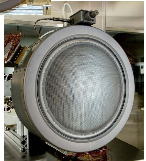
NEXT 6.9 kW Ion Engine
