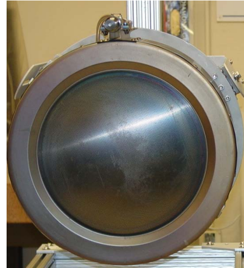
NSTAR 2.3 kW Ion Engine
