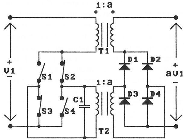
Figure 5. Full-bridge Complementary-resonant Converter.
