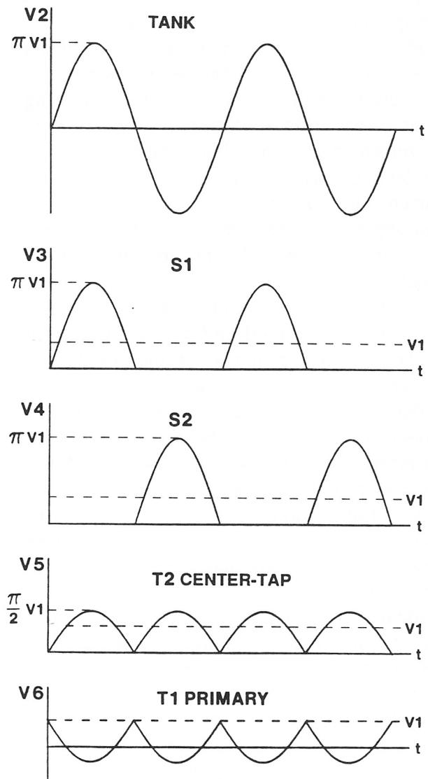
Figure 2. Ideal Waveforms For a Center-tapped Complementary-resonant Converter.
