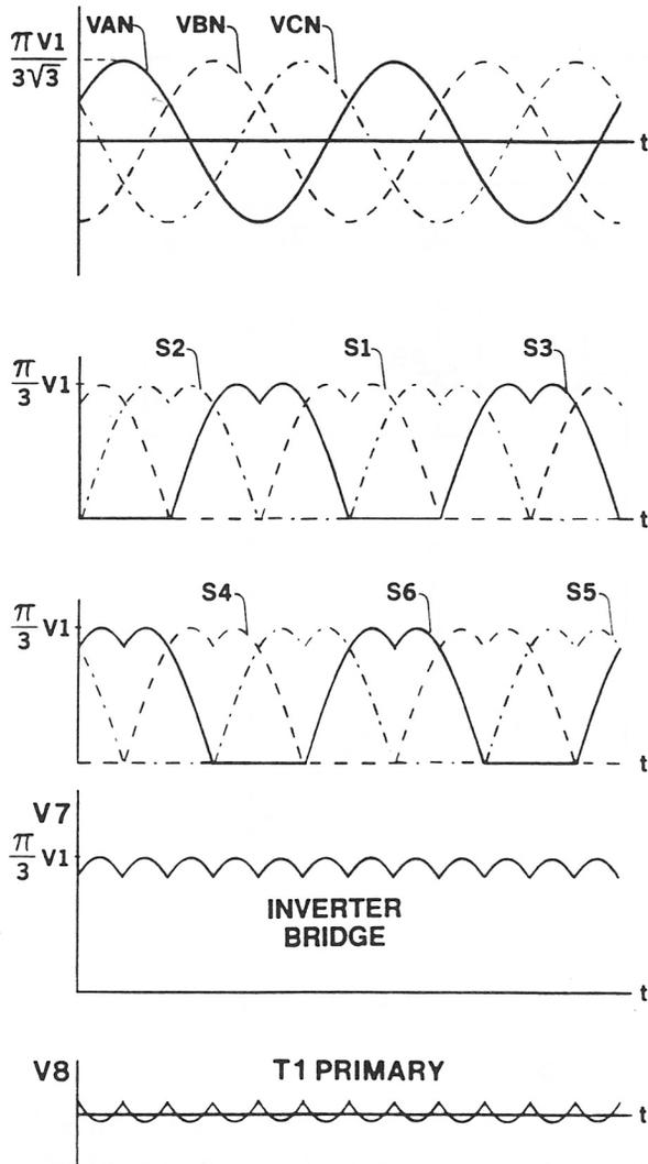
Figure 7. Ideal Waveforms For a Three-phase Complementary-resonant Converter.
