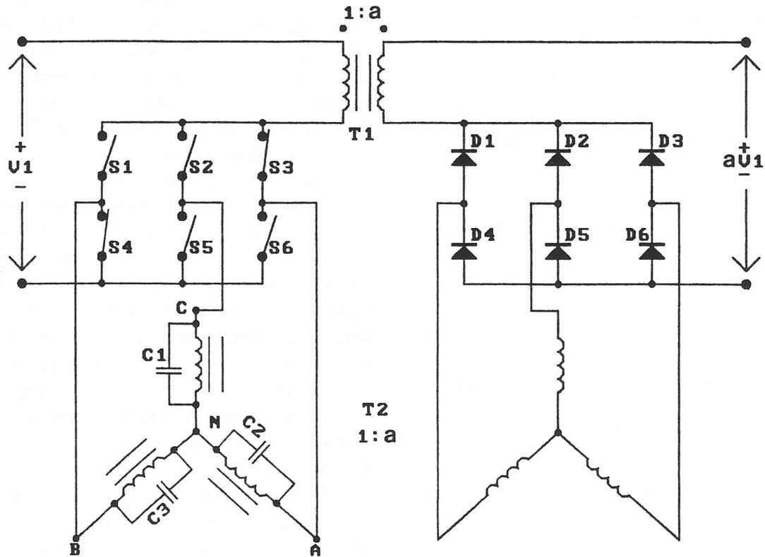
Figure 6. Three-phase Wye Complementary-resonant Converter.
