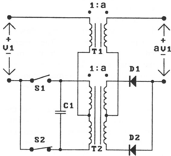
Figure 1. Center-tapped Complementary-resonant Converter.
